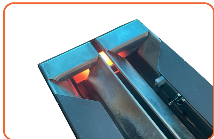
Figure. 4.5 PRIMING: Fuel is going to be ignited
